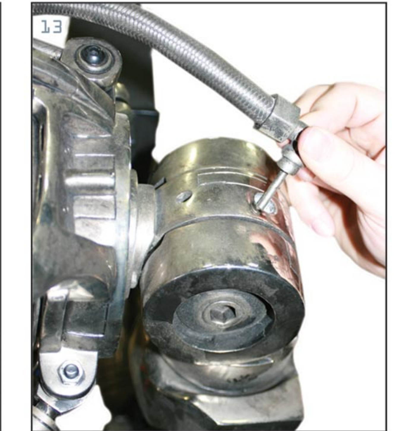
ATTACH CABLES (LEFT & RIGHT)
